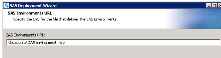
**SAS Environments URL:** The SAS environments file that is used by the SAS Cost and Profitability Management client application (and any other SAS clients that you install on this computer). The client application uses the environments file to locate other computers in your SAS deployment. Refer to [SAS 9.4 Intelligence Platform: Middle-Tier Administration Guide](#) for information about the SAS environments file.
